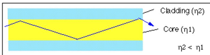
4. An optical fibre consists of a glass pipe coated with a second material of lower refractive index.
